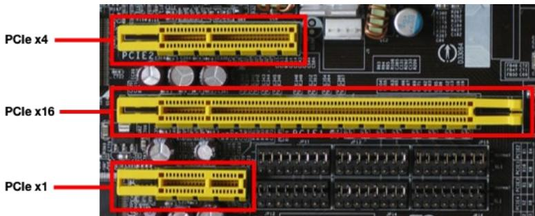
3. Now plug the PCIe-Host-Adapter-Card into a free PCI-Express slot. It does not matter if it is a x1, x4, x8 or x16 slot. After plugging in, you can now screw the plate of the PCIe-Host-Adapter-Card to the computer case.
